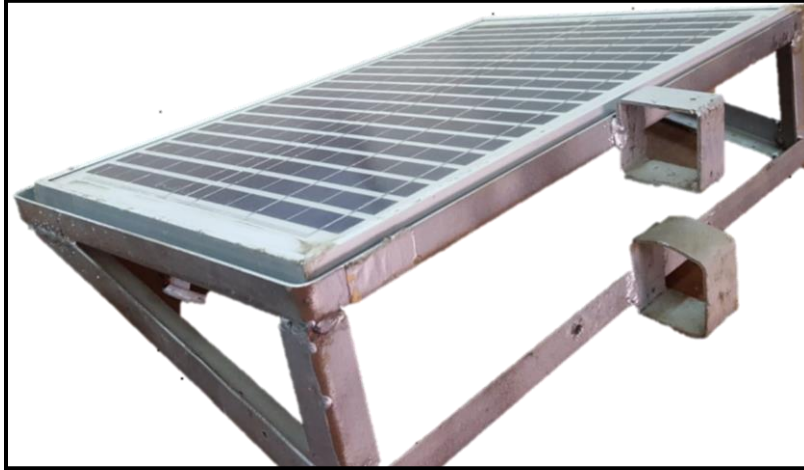
Figure 2. Mechanical housing with Panel
